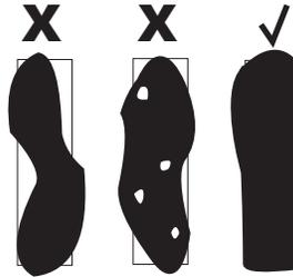
It may be necessary to adjust the position of the light source to maximize the contrast of the shadowline. Under normal conditions, optimal contrast is obtained by holding the instrument underneath and perpendicular to a light source.
