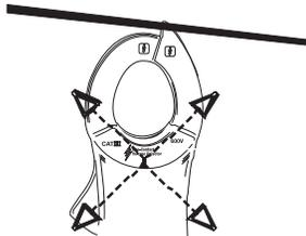
**NOTE:** The conductors in electrical cord sets are often twisted. For best results, move the probe tip along a length of the cord to assure placing the tip in close proximity to the live conductor.
