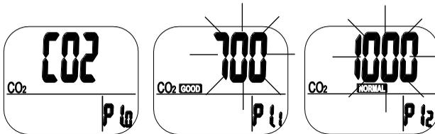
Press the ▲ or ▼ button to increase or decrease the value. Each press adjusts in 100 ppm increments. The range is 0 to 700 ppm (default is 700 ppm).
