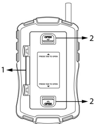
Opening tabs for battery compartment (1) and cable storage (2)
