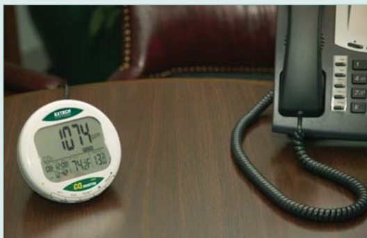
Desktop Carbon Dioxide (CO 2 ) Meter monitors the air quality in conference rooms insuring proper air ventilation
