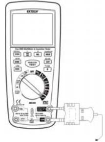
**Note:** The temperature probe is fitted with a type K mini connector. A mini connector to banana connector adaptor is supplied for connection to the input banana jacks.
